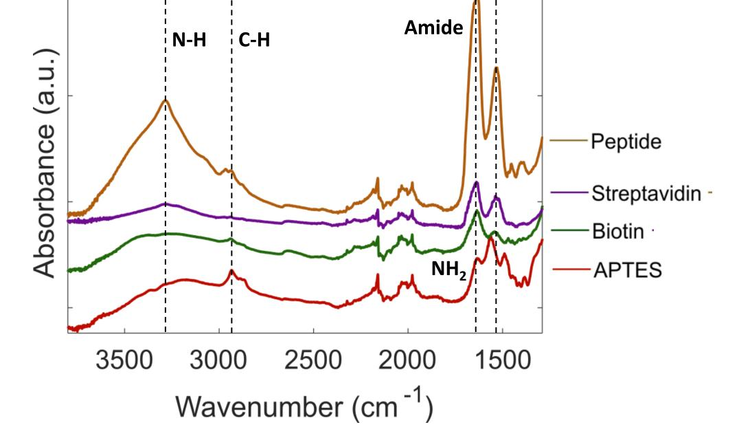
Expected peaks are present in the spectrum after each step, confirming each species was successfully attached to the PSi surface
