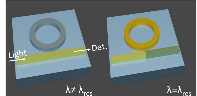
When  $\lambda \neq \lambda_{res}$ , all At  $\lambda_{res}$ , light light is transmitted through the waveguide to the detector.
