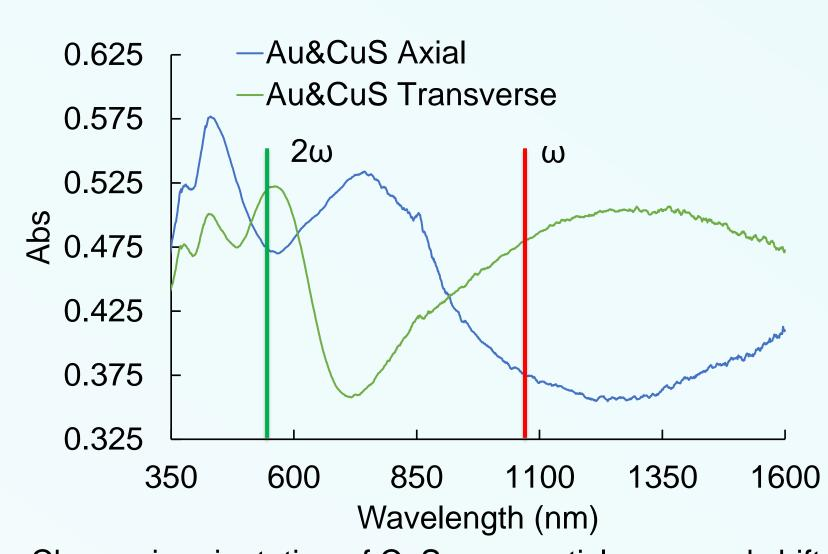
Change in orientation of CuS nanoparticles caused shift in LSPR peak due to change in which mode was excited (inplane vs out-of-plane)
