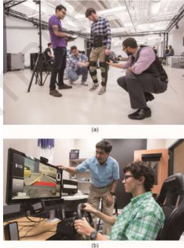
Fig. 1. Examples of Inclusion Engineering researchers at Vanderbilt University (photos courtesy of Vanderbilt University). (a) Researchers working on optimizing a lower body exoskeleton. (b) Driving simulator developed at Vanderbilt University to enable young adults on the autism spectrum to learn to drive. Monitors on the learning driver monitor physiological responses and attention to the road.
