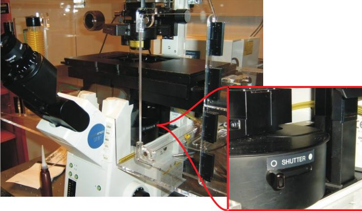
3. After the specimen is focused, the area of interest is selected, and fluorescence is confirmed, unclick the EpiLamp button.
