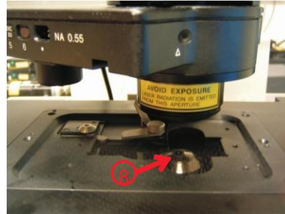
6. Mount the specimen on the stage. Remember that for inverted microscopes - those with the objectives below the stage - microscope slides must be placed upside-down.
