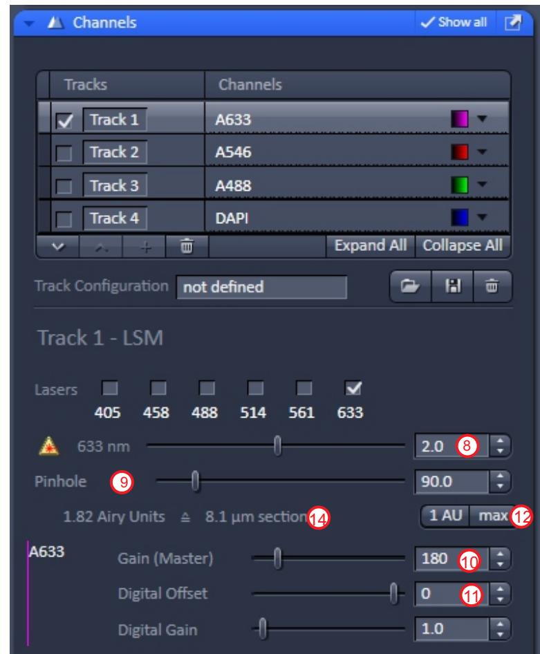
The pinhole size determines the thickness (Z dimension) of the sample from which light is gathered for the image. Larger pinhole size = more light reaching the PMT detector. However, a larger pinhole results in a "fuzzier" image.
