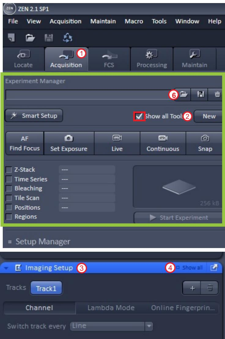
5. Create an imaging configuration that includes all of the excitation/emission settings needed for your fluorescent molecules. Use the “Smart setup” tool discussed in the next section or **load the same configuration used in a previously saved image**. To use an old config, open the image and click the “reuse” button ⑥ near the bottom of the screen below the opened image.
