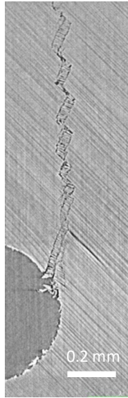
Figure 14. High magnification \mu CT tomograph of split/kink band in 45-degree ply (see Figure 13b). Voxel size is 2.55 \mu m.
