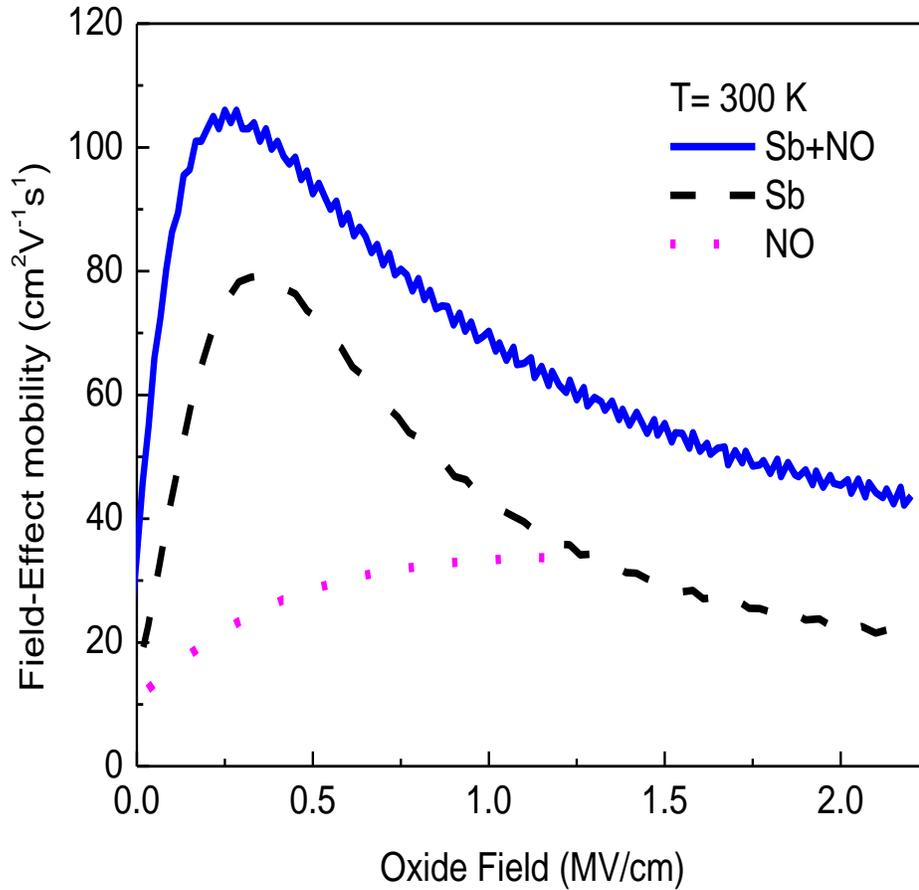
Figure 5. Field-effect mobility of 4H-SiC MOSFETs fabricated with three processes (i) NO: The standard method (ii) Sb: Antimony Counter-doping method (iii) Sb+NO: Combination of the two methods. Adapted from A. Modic, A.C. Ahyi, Y. Xu, P. Xu, M. Hamilton, Y. Zhou, L. C. Feldman, J. R. Williams and S. Dhar “High channel Mobility 4H-SiC MOSFETs by Antimony counter-doping”, *IEEE Electron Device Letters*, vol. 35, p. 894-896 (2014)
