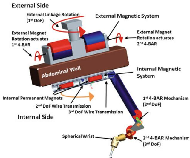
**Fig. 3** Schematic design of a surgical manipulator implementing 2 DoF by remote active magnetic actuation
