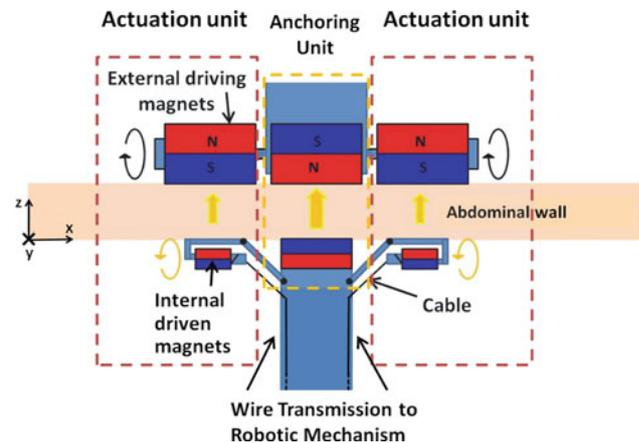
Fig. 2 Schematic design of remote active magnetic actuation. An anchoring unit and two rotational actuation units are combined to provide multiple DoF
