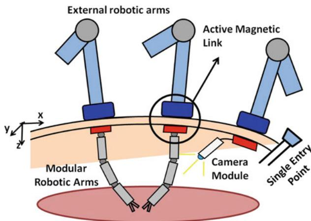
Fig. 1 Concept of the magnetically actuated surgical platform
