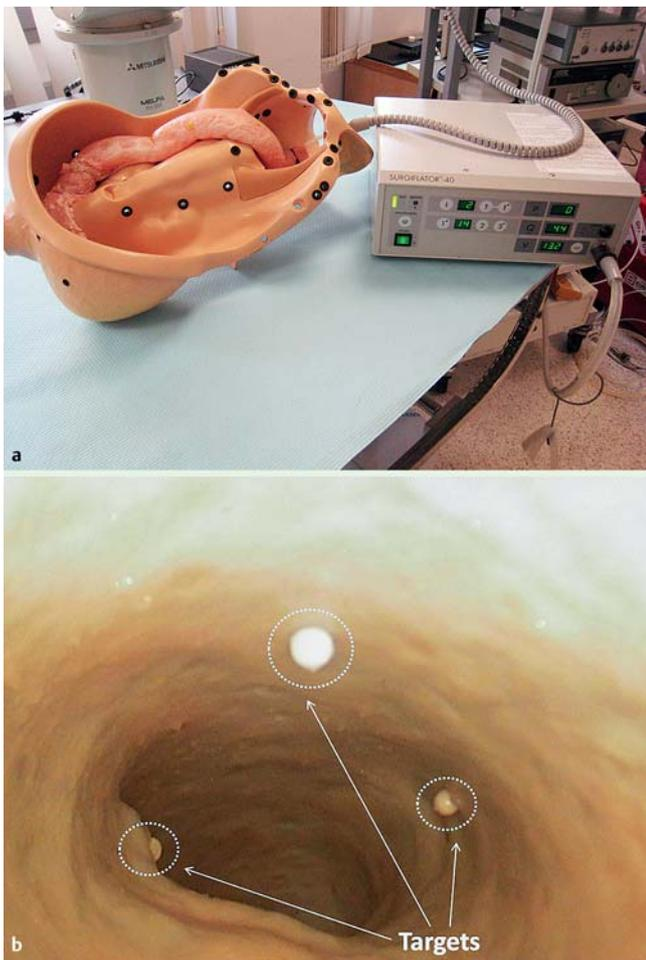
**Fig. 2** The lower gastrointestinal phantom model. **a** Colon tissue fixed inside the model. **b** Internal view of colon tissue with white spherical targets installed on the wall.
