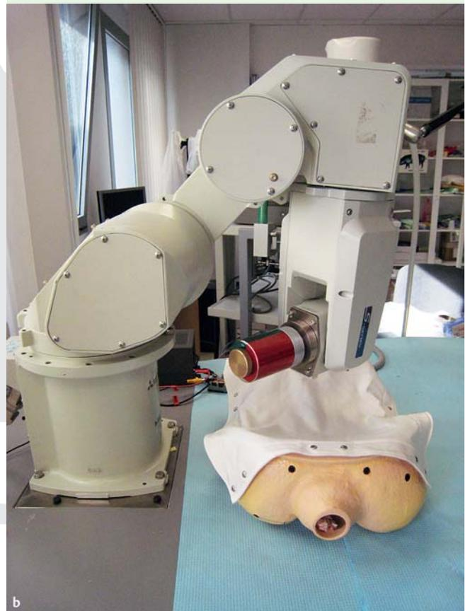
**Fig. 3** Movement of the external permanent magnet during the procedure. **a** Manual control; **b** robotic control. The colon simulator was covered by a dedicated layer in order to avoid a bias due to direct vision of the capsule inside the lower gastrointestinal simulator.
