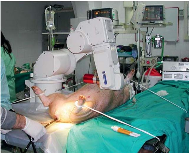
**Fig. 4** Test bench for magnetic capsule steering with the aid of a robotic arm in in vivo conditions.
