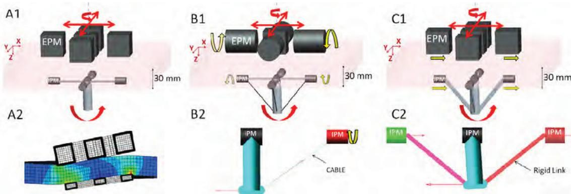
**Fig. 2 A1, B1, C1:** Schematic representations of PL, AMR and AMT approaches. **A2, B2, C2:** In A2 an ABAQUS FEA simulation of EPM-tissue-IPM interaction during a pitch displacement for the PL approach. In B2 and C2 ADAMS analysis of force/torque transmitted at the joint for the AMR and the AMT approaches, respectively.
