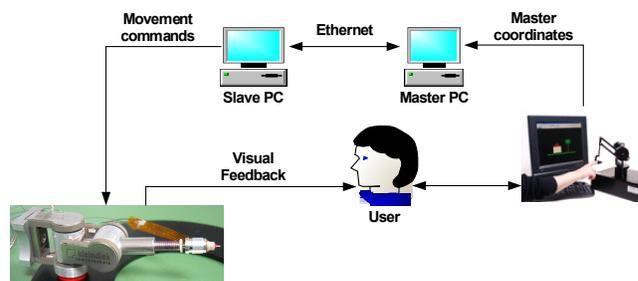
Fig. 2. The architecture of the teleoperated system.
