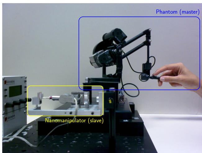
Fig. 1. The teleoperated system, highlighting the master and slave units.
