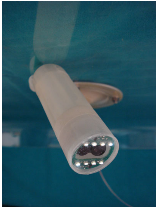
Fig. 7. Assembled prototype magnetically anchored to the abdomen simulator.
