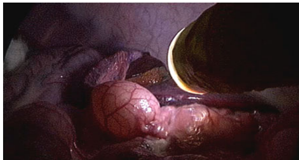
Fig. 12. Additional traditional laparoscope was inserted during the in vivo test to follow and evaluate the motion of the robot within the abdominal cavity. In the figure, the robot (on the right) is observing a section of the abdominal cavity (intestine and liver).
