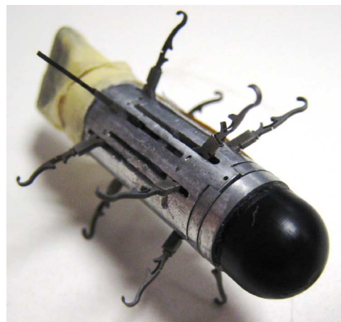
Fig. 9. Assembled 12-legged capsule. The black dome simulates the volume of a snap-on vision system for capsular endoscopy.
