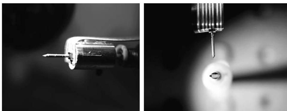
Fig. 3. The triaxial force sensing device mounted onto its aluminium support.
