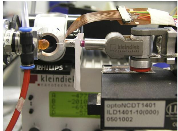
Fig. 9. Cell palpation and injection setup.
