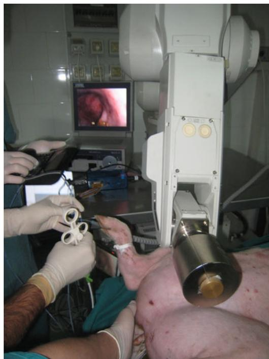
**Fig. 5** Setup for in vivo trials. A first operator was controlling the MAC, while a second one was using the polypectomy loop
