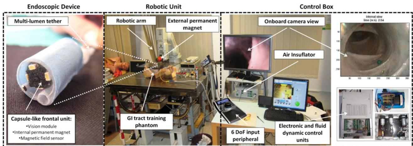
**Fig. 1** View of the complete endoscopic platform, consisting of the endoscopic device (*left*), the robotic unit (*center*), and the control box (*right*)
