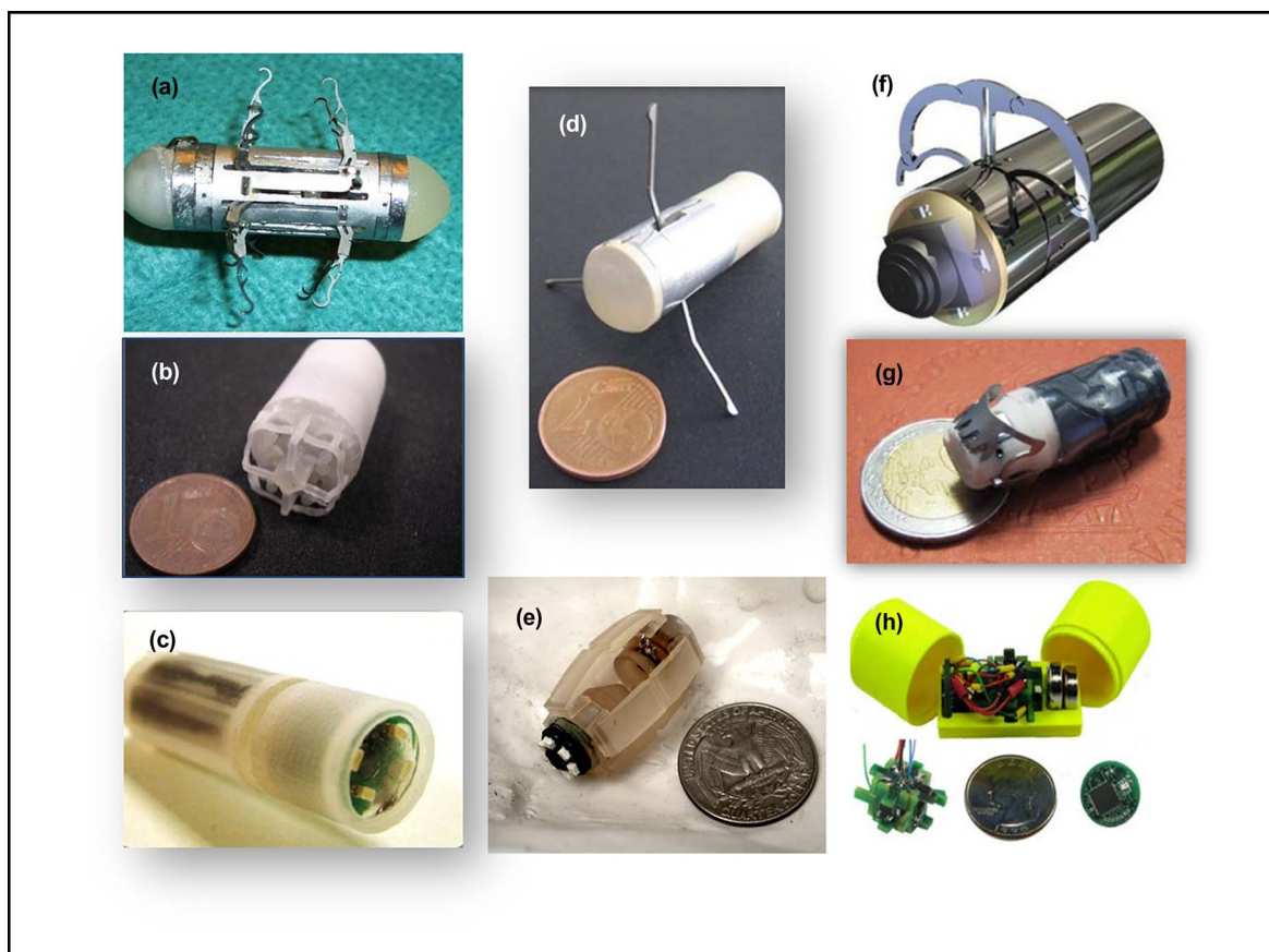
Figure 1. Selection of MCRs developed to date. Diameter and length of each prototype are provided in millimeters in parentheses: (a) 12-leg capsule [5] (11 × 30); (b) submarine-like capsule [6] (11 × 29); (c) magnetic capsule [7] (11 × 29); (d) legged-magnetic hybrid capsule [8] (14 × 38); (e) magnetically actuated capsule endoscope (MASCE) [9] (15 × 40); (f) drug delivery capsule [10] (11 × 25); (g) surgical clip releasing capsule [11] (11 × 30); and (h) magnetic capsule with localization [12] (11 × 26).
