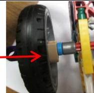
Make sure the rubber band holder (purple) is centered on the axle (rotating shaft connecting wheels)
